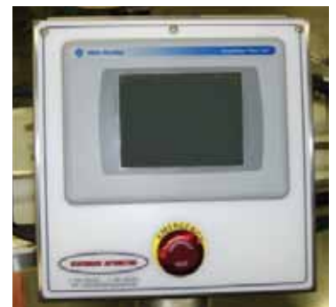
Color touch screen operator interface allows slug length changes while running or by recipe selection.
