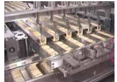
Independent measuring pins gently enter the continuous lanes of on-edge product.
