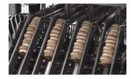
Servo control allows for slug length changes to be made using the machine's HMI and without any changeover parts.
