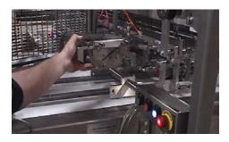
Bucket changes are made quickly, easily and without the need for any tools.
